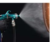
Each gun can be configured with the appropriate needle and nozzle to accommodate the coating, size of part and type of surface to be finished.
